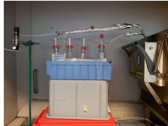
Strictly tubular reactor, filled with charcoal, mounted in a muffle oven and spilled by activation gas at a certain temperature for a set period of time
