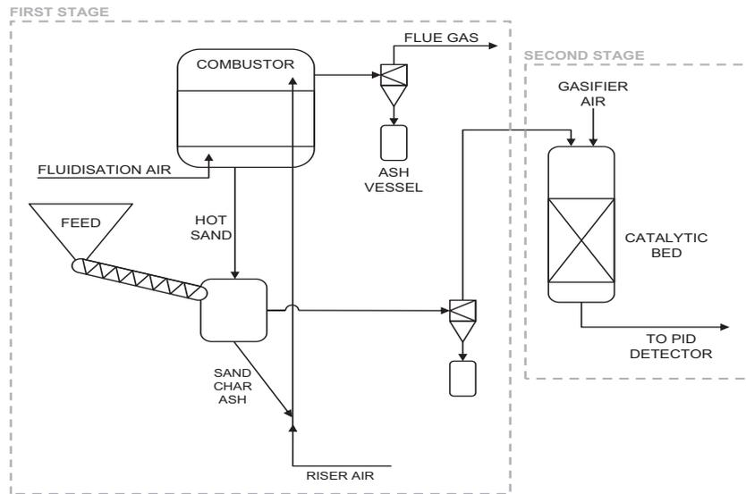
Schematics of the tar measurement system for real gas tests at BTG
