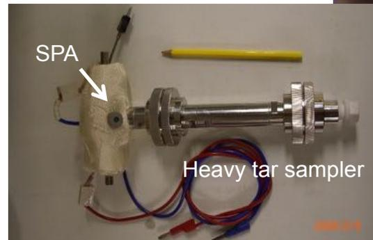
Sampler mounted on atmospheric fluidised bed gasifier
