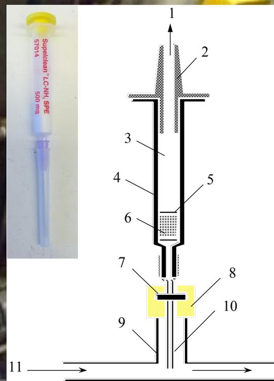
1 = to syringe or electrical pump; 2 = adapter (polypropylene); 3 = sample reservoir; 4 = sorbent tube (PP, 1.3 OD x 7.5 cm); 5 = fritted disc (20 mm polyethylene); 6 = amino-phase sorbent (40 mm, 60 Å); 7 = rubber/silicone septum; 8 = septum retainer (polypropylene); 9 = "Tee"-adaptor (glass); 10 = syringe needle (stainless steel); 11 = producer gas.
