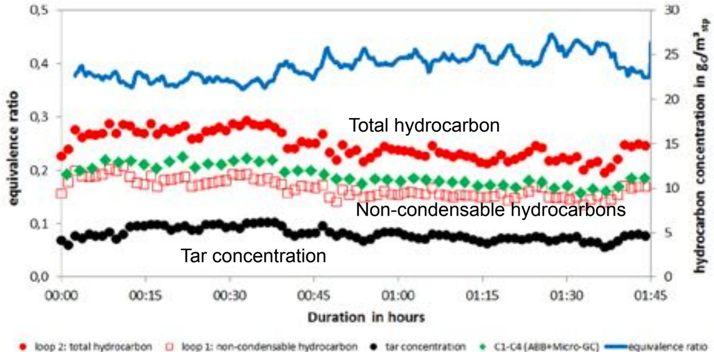
Fig. 9 Results of first field test with real producer gas from gasification
